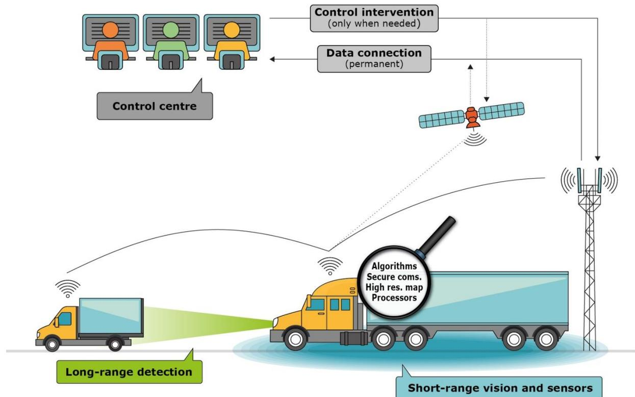
The three main components of a fully automated truck’s potential operating environment are its on-board systems, supporting infrastructure and the (remote) control centre. As noted above, fully autonomous vehicles would require less supporting ICT infrastructure, but that puts much stronger emphasis on the on-board systems.
