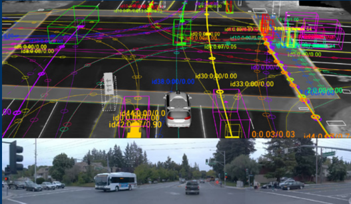
The simulated imagery shown demonstrates how our software assigns predictions to each object surrounding our vehicle—other vehicles, cyclists, pedestrians, and more.
